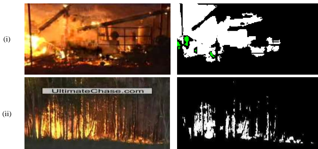
Figure 5. (a) Input video frames; (b) Output of fire regions with centers/no center (continued...)
